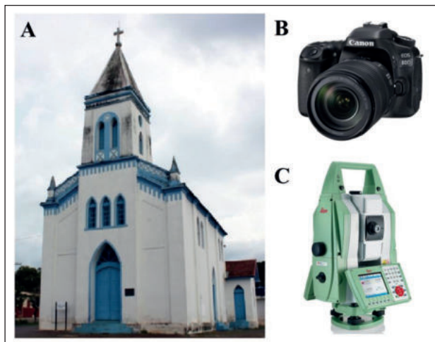
Figure 1 A Nossa Senhora do Rosario Church B Camera Canon 600D C Total Station Leica MS-50 with Laser Scanning
