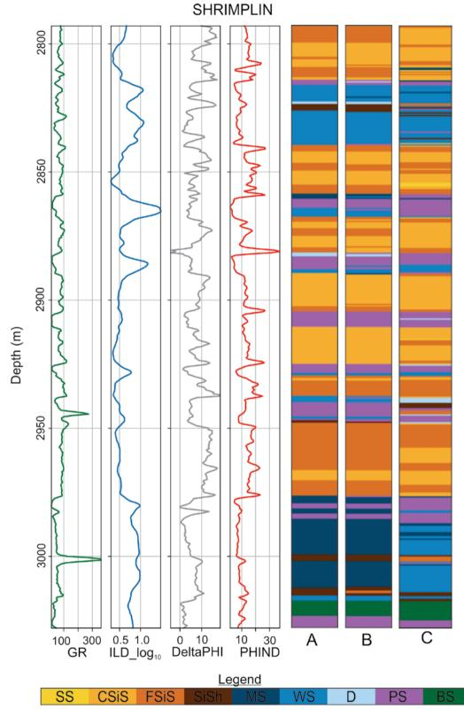
**Figure 8** A. Comparison between real facies; B. Facies predicted by t-SNE+K-NN; C. Facies predicted with the Dubois *et al.* (2007) ANN in the SHRIMPLIN well. There are also illustrated the gamma ray curves (GR), resistivity on a logarithmic scale on a base 10 basis (ILD\_log<sub>10</sub>), the difference between porosity and neutron density (DeltaPHI) and the average porosity and the neutron density (PHIND).
