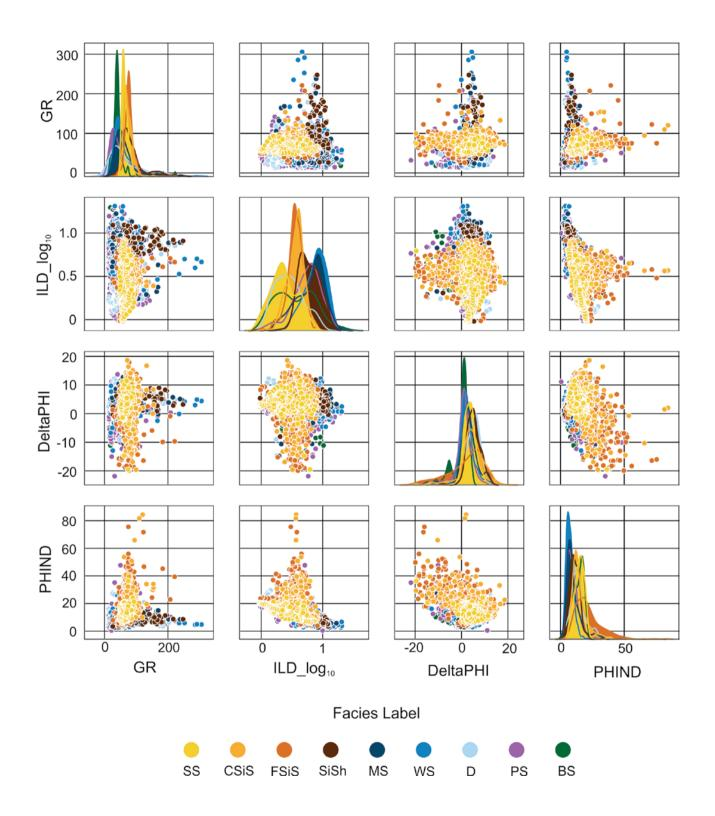
**Figure 3** Bivariate diagrams for evaluating the behavior of the measured properties (GR, ILD\_log<sub>10</sub>, DeltaPHI and PHIND) in each of the nine facies. The facies are represented by colored dots that form a cloud where the boundaries between facies cannot be defined due to overlapping data.
