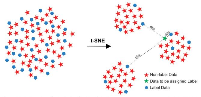
Figure 2 Methodology adopted for classification of geological facies. The stars and pentagons represent non-labeled and labeled samples, respectively. For a given non-label sample (green star) is computed the Euclidean distance regarding each labeled sample, and the labeled is assigned according to the samples with lower distance (K-NN method).
