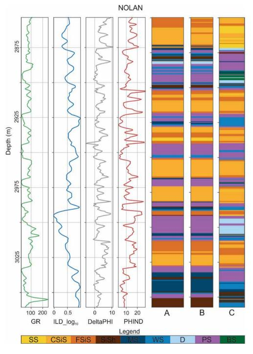
**Figure 7** A. Comparison between real facies; B. Facies predicted by t-SNE+K-NN; C. Facies predicted with the Dubois *et al.* (2007) ANN in the NOLAN. There are also illustrated the gamma ray curves (GR), resistivity on a logarithmic scale on a base 10 basis (ILD\_log<sub>10</sub>), the difference between porosity and neutron density (DeltaPHI) and the average porosity and the neutron density (PHIND).
