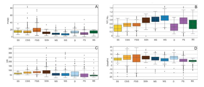
**Figure 4** BoxPlot diagrams in which it can be observed the overlap in the space of the measured properties for each of the facies; A. PHIND; B. ILD\_log<sub>10</sub>; C. GR; D. DeltaPHI. Facies are represented by colored rectangles that show the variation of the measured data and the points scattered by the diagrams represent the outliers in each variation.
