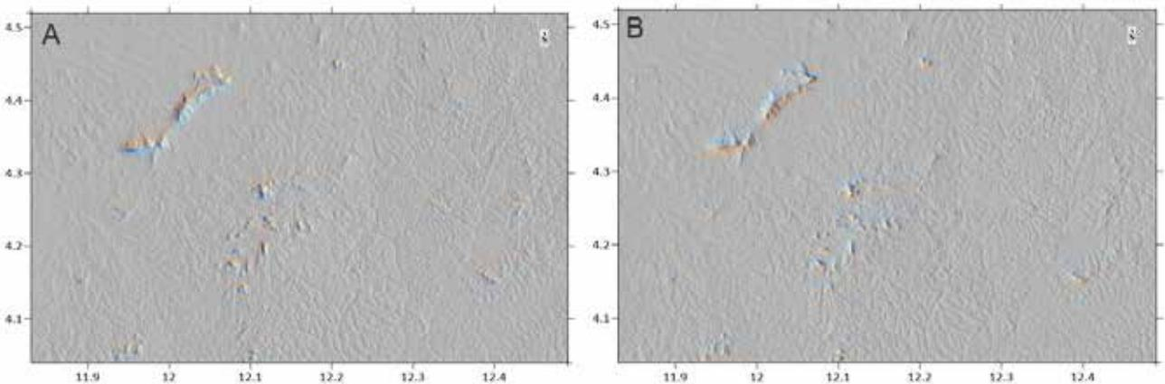
Figure 5 Two shaded relief images created by combining different shaded relief images; A. Combining four shaded relief images with sun angle of  $0^\circ$ ,  $45^\circ$ ,  $90^\circ$  and  $135^\circ$ ; B. Combining four shaded relief images with sun angle of  $180^\circ$ ,  $225^\circ$ ,  $270^\circ$  and  $315^\circ$ .
