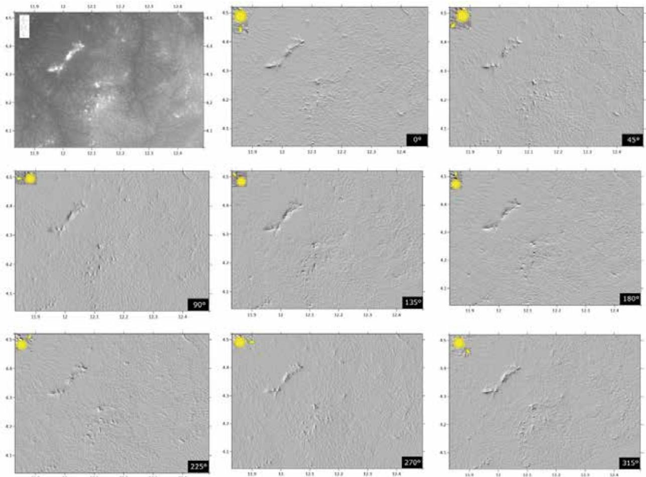
Figure 4 Hill-shaded images with a constant light dip of  $45^\circ$  and various light azimuths, covering part of the study area (blue rectangular box in Figure 3). The yellow arrows in each hill shaded DEM represent the direction of the Sun Azimuth.
