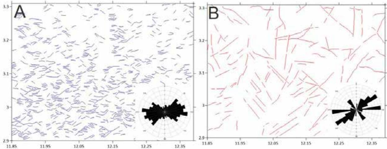
Figure 8 A. Lineament maps of Sangmelima area obtained from automatic extraction of remote sensing images; B. and compared to those extracted from the geological map (see Figure 1C)
