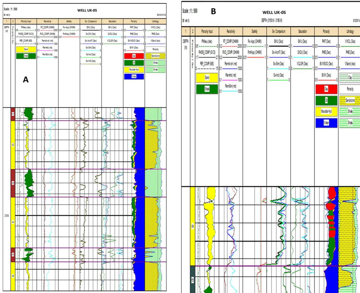
**Figure 7** A. Wireline log for Well UK-05 with interpreted lithology showing alternation of sands and shales with the fluids saturating the reservoirs being gas, oil and water; B. Wireline log for Well UK-05 with interpreted lithology showing alternation of sands and shales with the fluids saturating the reservoirs being gas, oil and water
