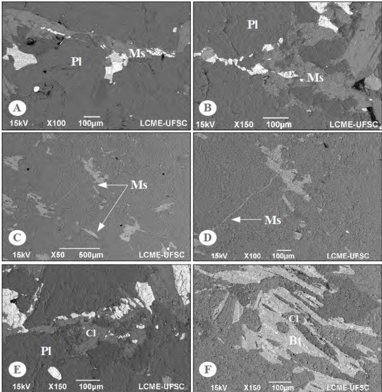
**Figure 8** BSE images of tonalitic gneiss: A-B. Fractures in plagioclase crystals (Pl) in filled with white mica (Ms); C. Small fractures filled with secondary material; D. Detail of small fractures with filling of secondary material; E. Chlorite (Cl) filling cracks in plagioclase; F. Partial alteration from biotite (Bt) to chlorite (Cl) along the cleavages.
