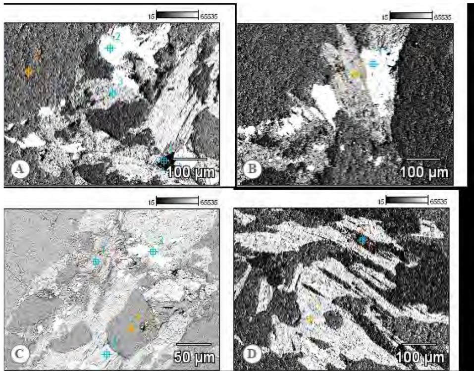
**Figure 9** BSE images of tonalitic gneiss: A. Biotite altered to chlorite (1) chlorite (2) iron oxide (3) biotite (4) plagioclase; B. Biotite altered to chlorite (1) hematite (2) biotite altered to chlorite; C. Process of alteration from biotite to chlorite (1) chlorite (2) biotite altered to chlorite; D. Localized occurrence of chlorite and white mica along biotite cleavages (1) chlorite (2) white mica (3) iron oxide (4) quartz.
