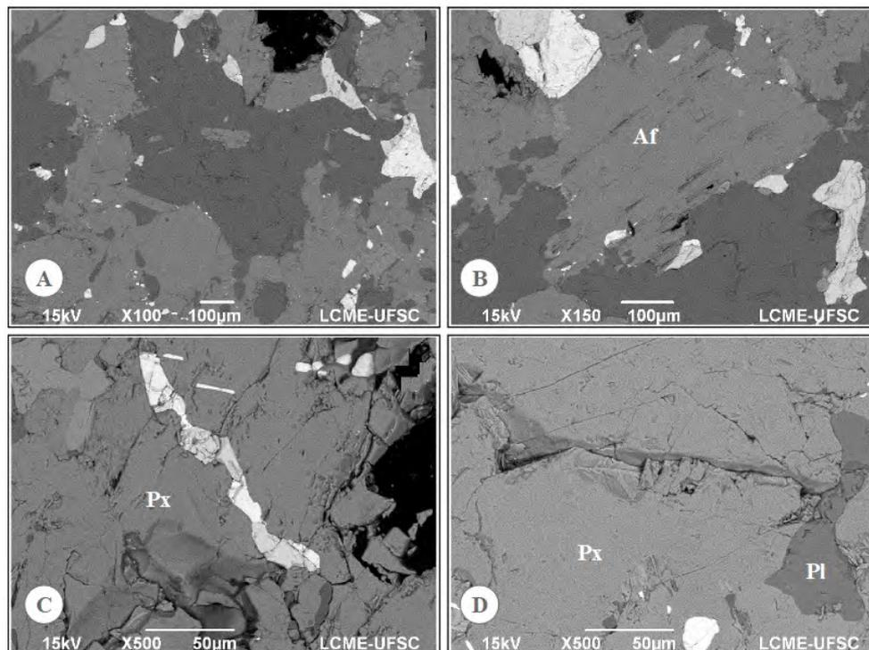
**Figure 10** BSE images of the enderbitic gneiss: A. Thin fractures in plagioclase crystals with no filling by alteration material; B. Amphibole crystals without fractures; C. Transgranular fractures in pyroxene crystals without secondary filling; D. Grooves and fractures in pyroxene crystals without secondary filling, as well as the occurrence of pyroxene and plagioclase.
