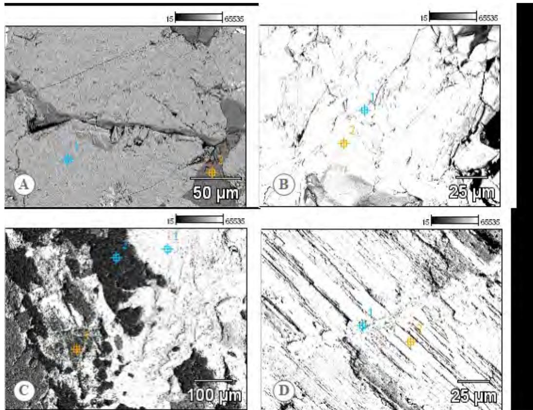
**Figure 11** BSE image of the enderbite gneiss: A. Pyroxene crystal with transgranular fractures and without secondary filling (1) pyroxene (2) plagioclase; B. Biotite partially replaced by Fe-Ti oxides (1) and chlorite (2); C. Alteration zone filled with white mica+quartz near the contact between quartz crystal and chlorite (1) biotite (2) quartz (3) white mica; D. Chlorite filling (1) in biotite fracture (2).
