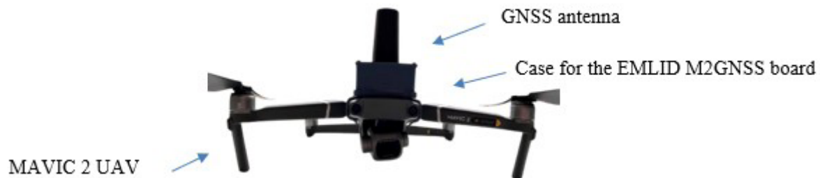
Figure 4 The mounting case for the receiver and the antenna.
