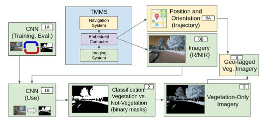
Figure 2 The workflow: 0 is data acquisition; 1 is the use of the CNN; 2 to 4 is the remaining part aiming to the final product.
