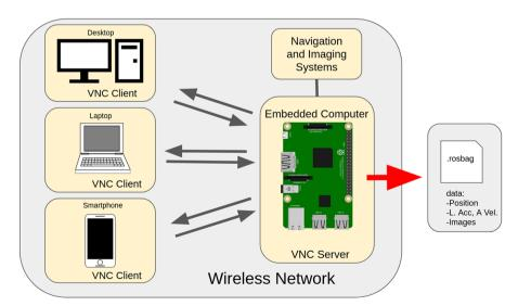
Figure 3 The Platform Control Scheme.
