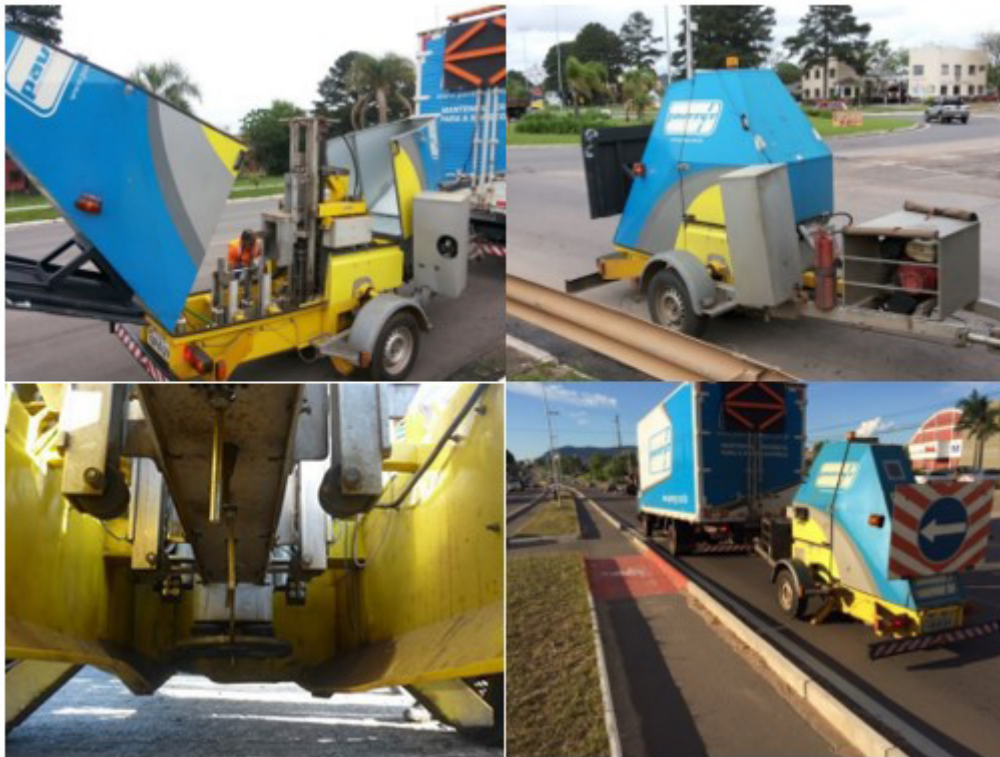
Figure 1 FWD equipment used to perform the deflectometric tests.
