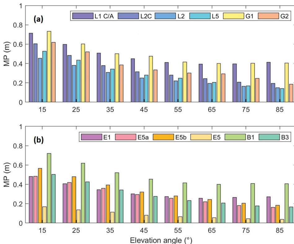
Figure 2 MP index versus elevation angle for: A. GPS and GLONASS signals; B: Galileo and BeiDou signals.
