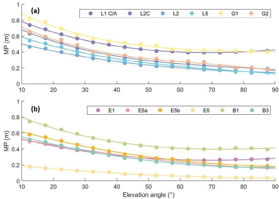
**Figure 3** MP observations (dots) and modeled function (continuous lines), considering the elevation angle and signals from: A. GPS and GLONASS; B. Galileo and BeiDou.
