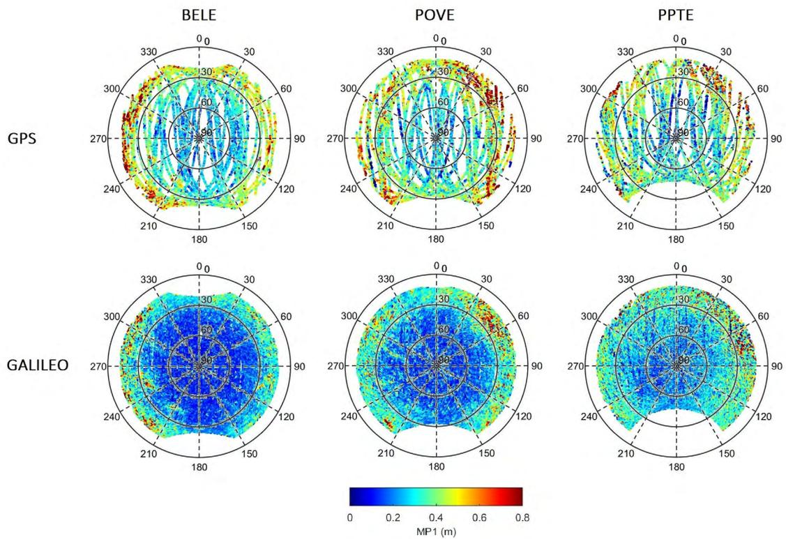
Figure 5 BELE, POVE and PPTE stations sky-plot, considering GPS and Galileo satellites.
