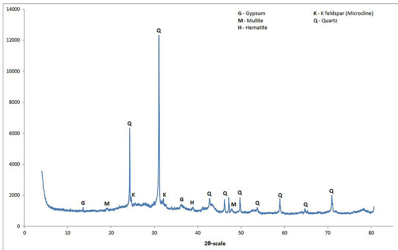
Figure 7 The x-ray diffractogram (Cock) of roof tile sample.
