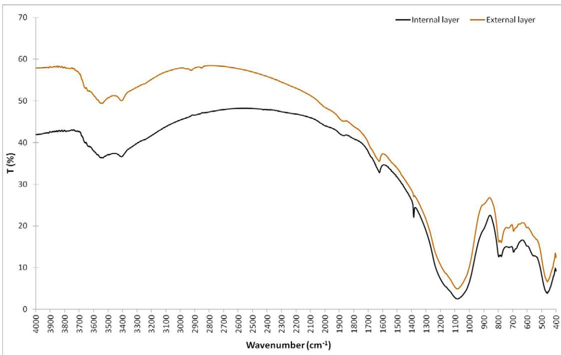
Figure 9 Fourier transform infrared spectroscopy (FTIR) of roof tile sample.
