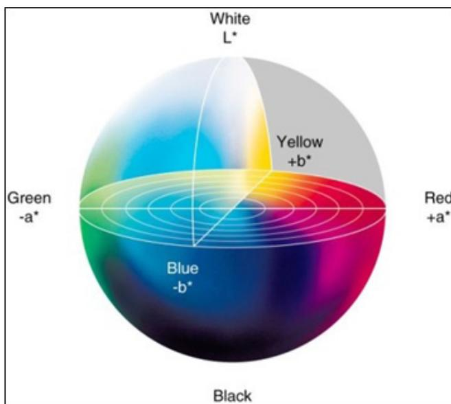
Figure 4 The CIELAB color space representing in three color coordinates  $L^*$ ,  $a^*$  and  $b^*$  (Eissa et al. 2013).
