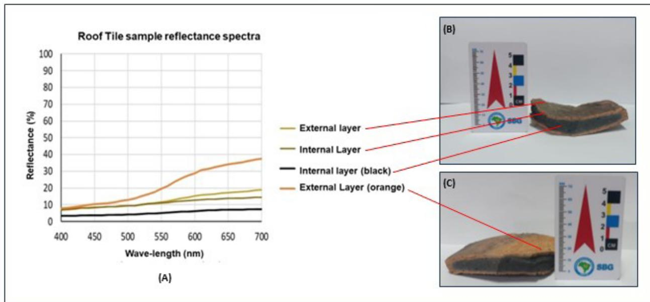
Figure 10 The differences between patterns L\*, a\* and b\* for the roof tile sample: A. Reflectance Spectra Sample; B. Concave position of the roof tile sample; C. Convex position of roof tile sample.
