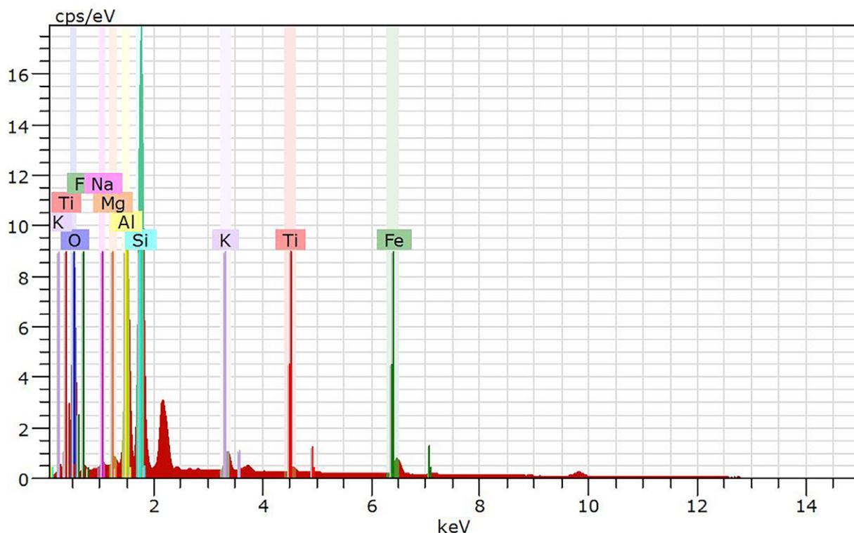
Figure 8 Scanning Electron Microscopy with Energy Dispersion (SEM-EDS) of the internal roof tile sample.
