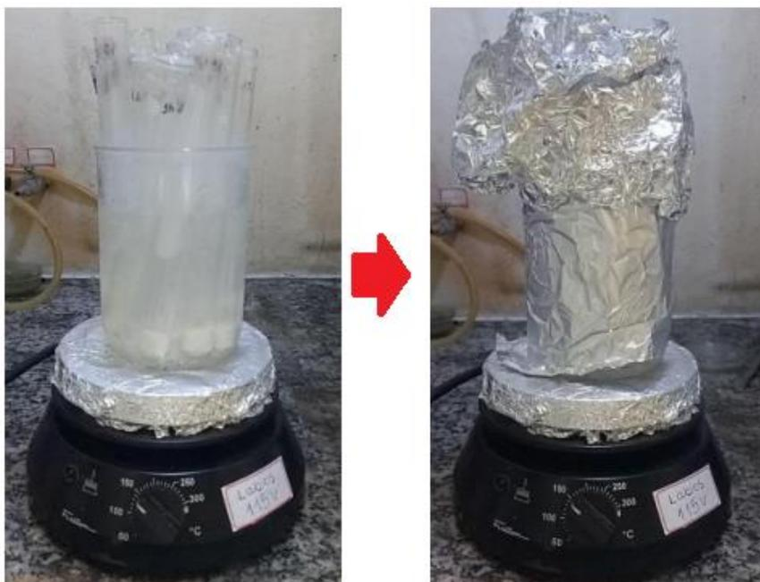
Figure 1: Synthesis of multiple Bio-PCM samples.
