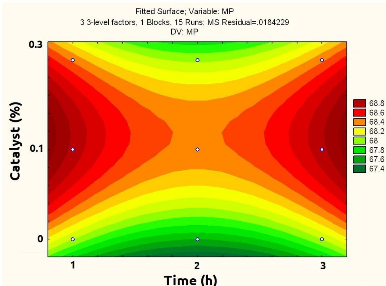
Figure 3: Correlation between the catalyst percentage and the reaction time.
