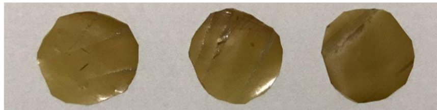
Figure 1. The visual aspect of cassava starch biofilms with aqueous extract of C. guianensis
