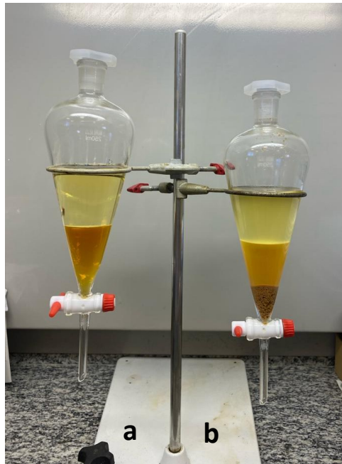
Figure 1: biodiesel synthesis: Homogeneous catalysis (a) and heterogenous catalysis (b)
