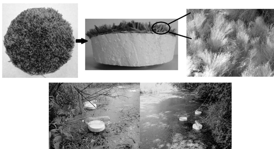
Figure 2. Artificial substrate sampler made of polyester carpet and experimental design with the position of artificial substrate samplers on the margin of Guareí River, State of São Paulo, Brazil.
