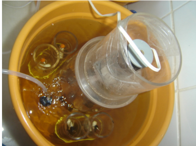
Figure 2. Picture of the schematic incubation system showing the aquarium with water and sediment samples from Baía das Pedras during the stabilization time.
