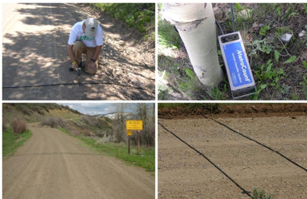
**Figure 2.** Images of a pneumatic counter, clockwise from top left: author installing pneumatic tube on the road surface; battery-powered electronic monitoring device; parallel pneumatic tubes across the road; typical view of a pneumatic counter across a road in the study area.
