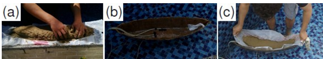
Figure 6: (a) Preparation of the argil mass; (b) Measurement with the empty boat; (c) Measurement with a distributed mass of 2 kg.
