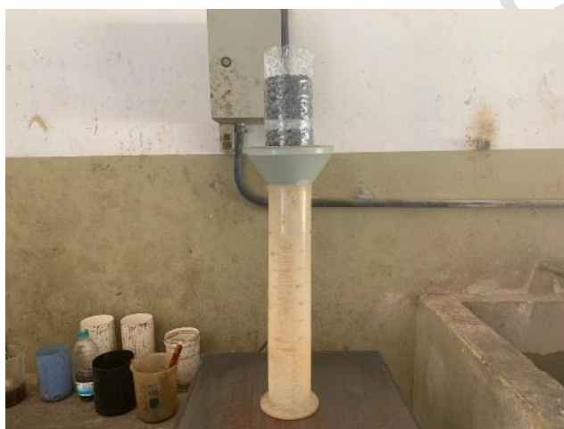
Figure 3: ISO 17785-1 infiltration rate test setup
