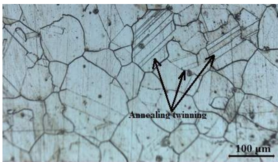
Figure 1: Microstructure of commercially Inconel 625 Ni-based superalloy.
