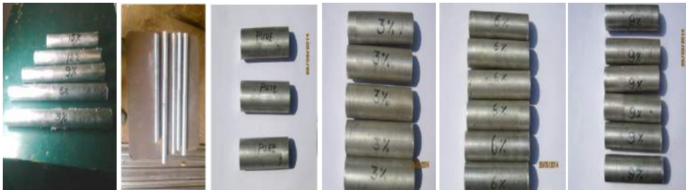
Figure 2: Cast samples of LM25-ZrO 2 composites
