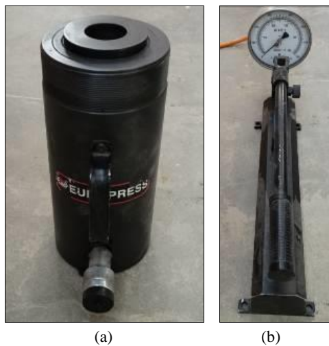
Figure 3: (a) Hydraulic jack and (b) manual pump for service load application.
