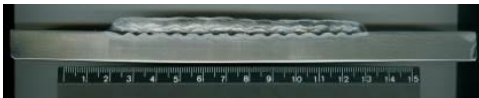
Figure 2: Macrography of the weld overlays. Etching: Aqua Regia.
