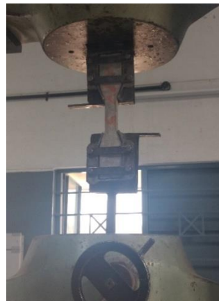
Figure 4: Dog bone specimen under direct tensile load.
