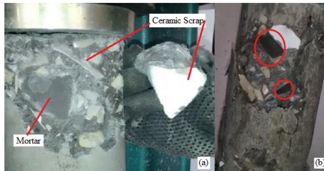
Figure 5: Ceramic scrap/mortar interface rupture model in the concretes: (a) CSC-III; (b) CSC-II.
