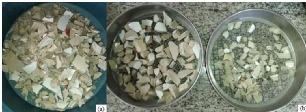
Figure 1: Granulometric distribution tests: (a) ceramic scrap sample to granulometric distribution; (b) sieves.
