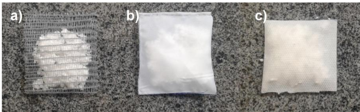
Figure 2: Specimens for sorption assay with envelopes of: a) polypropylene; b) polyester and c) polypropylene
