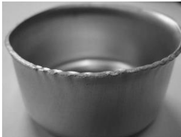
Figure 11: Piece drawing with a Teflon film.
