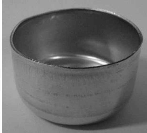
Figure 10: Piece drawn in which wrinkling does not occur.
