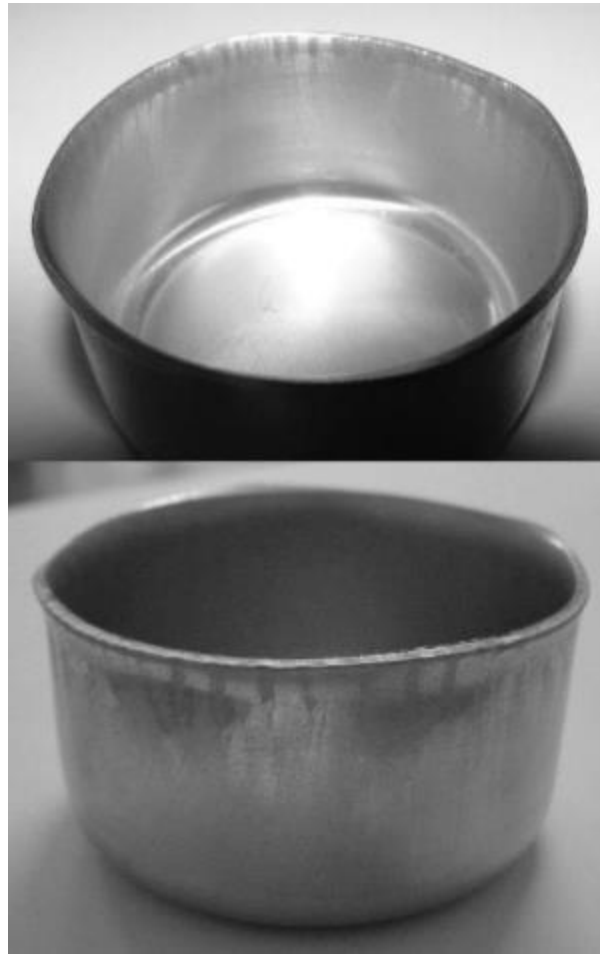
Figure 12: Piece drawing with grease lubricant.
