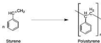
Figure 1: Chemical structure of Polystyrene. The polymer is a repetition of units of styrene.
