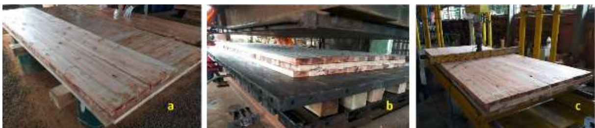
Figure 9: Manufacture of Eucalyptus CLT panel, a) assembly and application of adhesive, b) panel pressing, and c) panel finalized during bending test in laboratory. Source: Author
