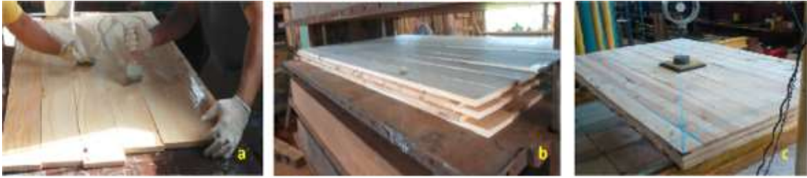
Figure 10: Manufacture of Pinus CLT panel, a) assembly and application of adhesive, b) panel pressing, and c) panel finalized before test in laboratory. Source: Author
