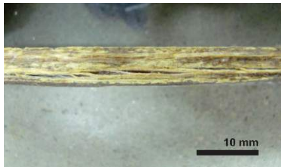
Figure 4: Lateral view of a phenolic composite specimen after 71 days of alkaline exposition.
