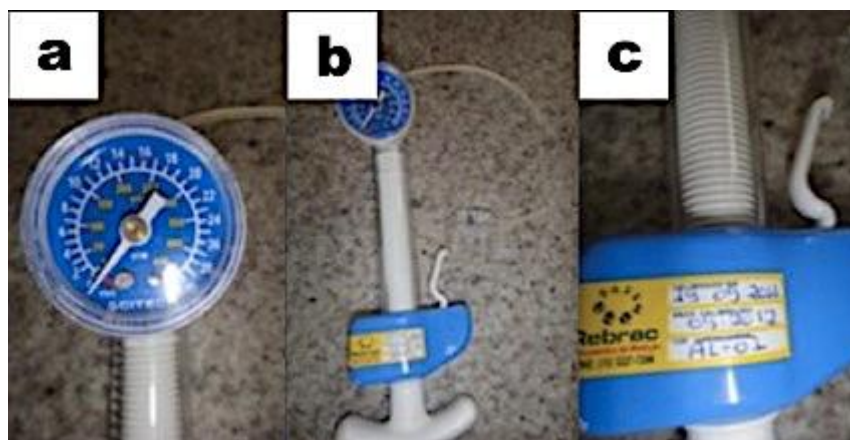
Figure 3: Inflation syringe: (a) Gauge, (b) Front view of the inflation syringe, (c) Calibration certificate.
