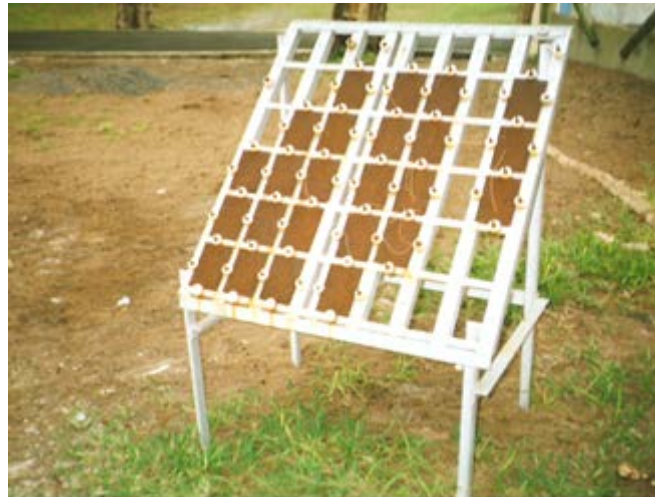
Figure 2: Exposure of carbon steel samples on exposure racks
