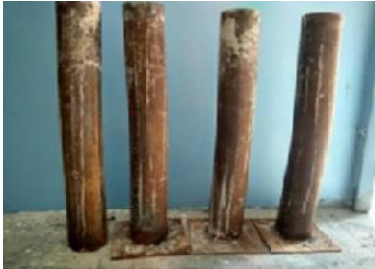
Figure 14: Behavior of CFST Column after Axial Load.
