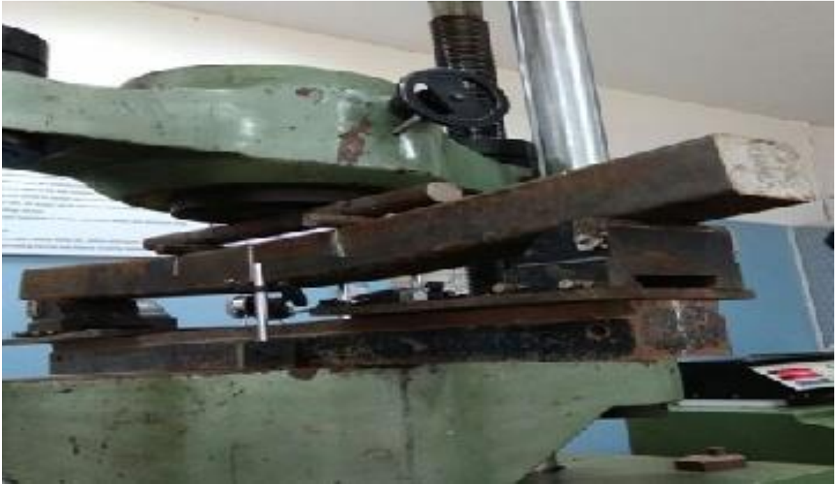
Figure 11: Typical Flexural behavior of CFST beam under flexural Loading.
