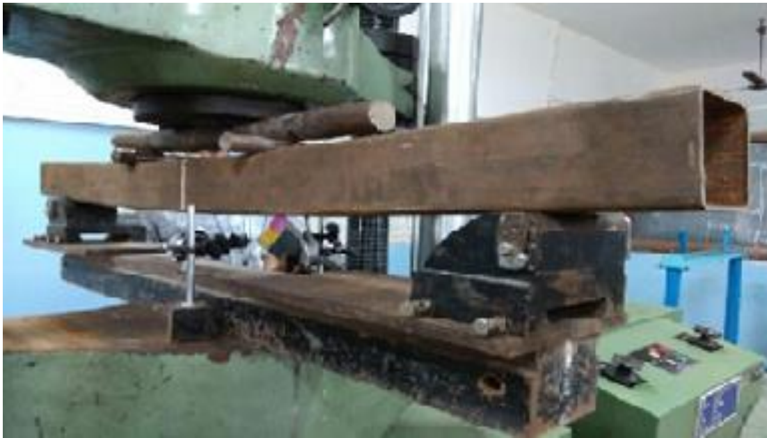
Figure 2: Flexural Load Setup of CFST Beam.
