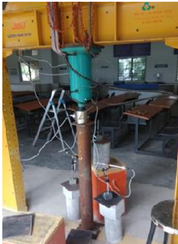
Figure 2: Flexural Load Setup of CFST Beam.
