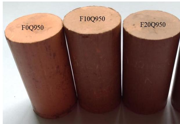
**Figure 5:** Tests pieces burned at 950°C with 0, 10 and 20% of waste.
