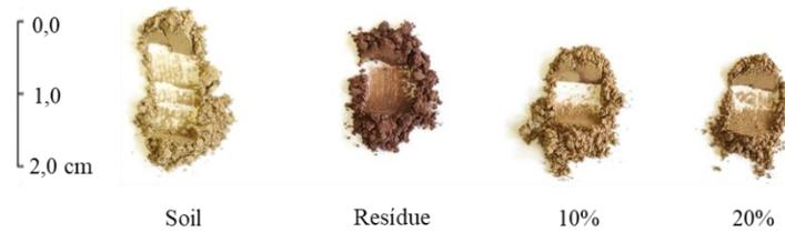
**Figure 1:** Samples of the soil, the residue and the formulations with 10 and 20% of residue.
