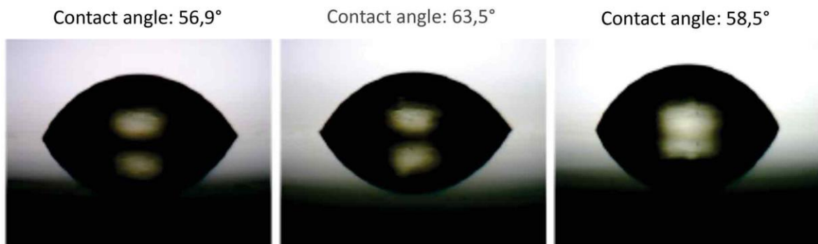
Figure 6: Contact angle image on three different areas of the anodized sample.
