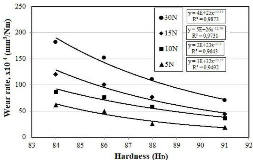
Figure 6. Relationship between hardness and wear rate of the composites in the inserts.
