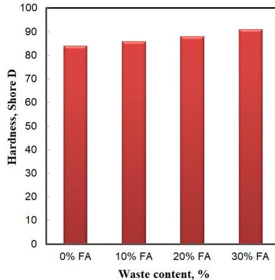
Figure 2. Hardness of FA polymer composites
