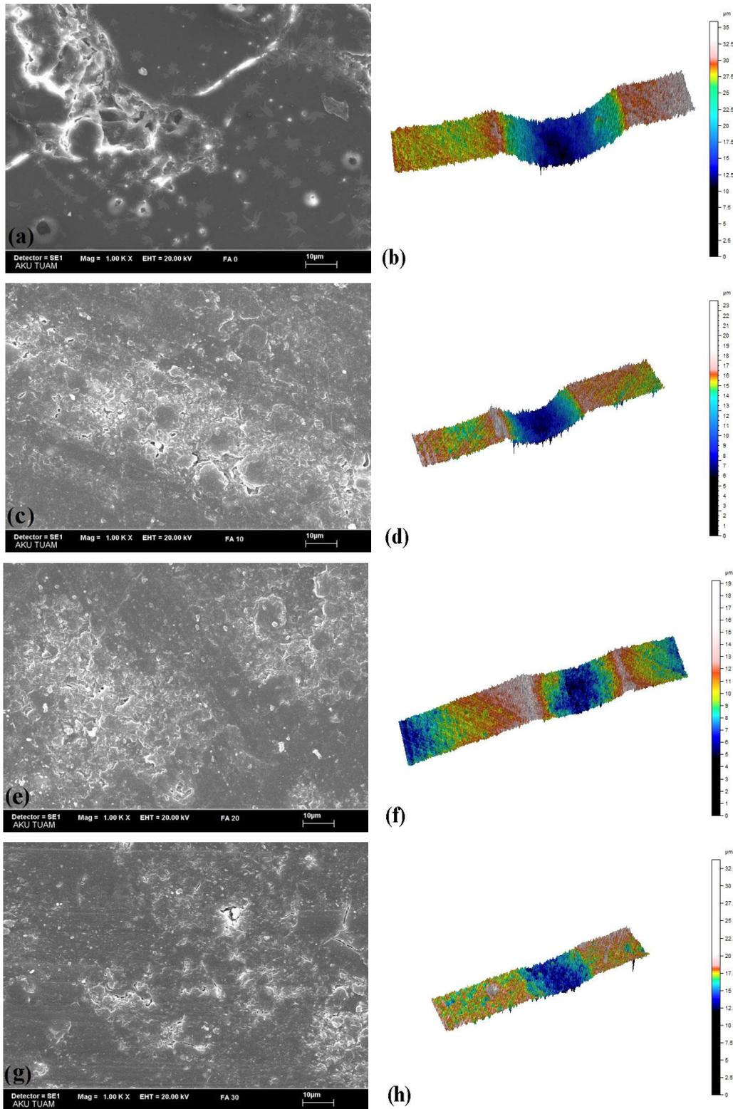
**Figure 9.** SEM micrograph and cross-sectional surface of the worn-out surfaces of epoxy composites after tribometry for various FA content: (a) for pure epoxy, (b) for pure epoxy CS, (c) for 10% FA, (d) for 10% FA CS, (e) for 20% FA, (f) for 20% FA CS, (g) for 30% FA, (h) for 30% FA CS.
