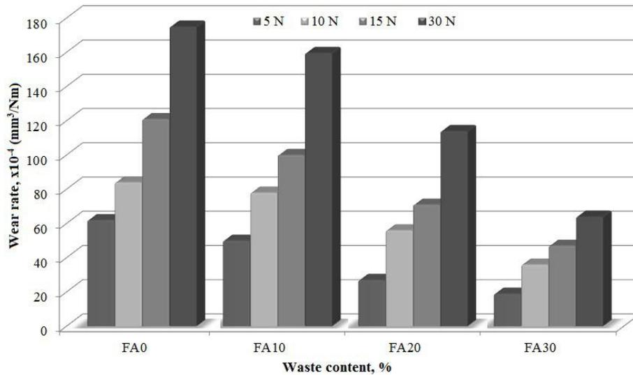
Figure 5. Wear rate of polymers depending on fly ash content.
