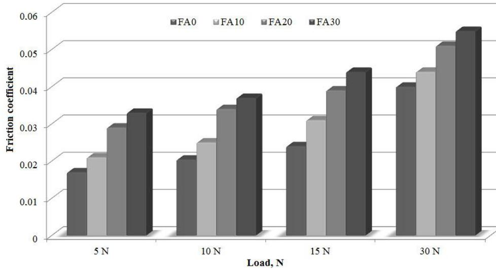
Figure 4. The variations in the friction coefficient values of polymer composites with fly ash.
