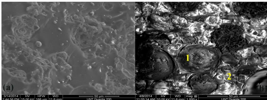
**Figure 1.** SEM micrograph of FA polymer composites: (a) 10% FA, (b) 30% FA matrix / fly ash.
