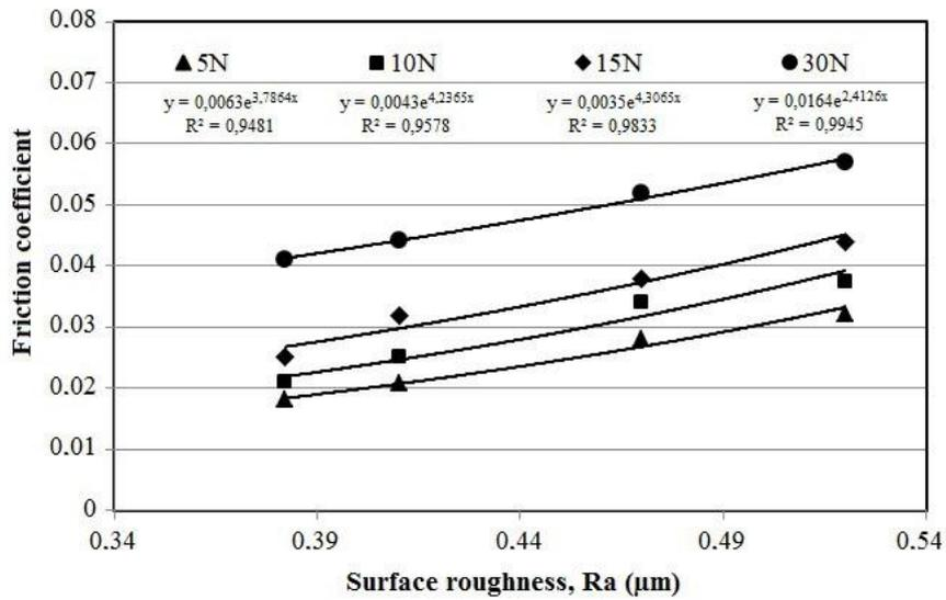
Figure 7. Relationship between dynamic friction and surface roughness.
