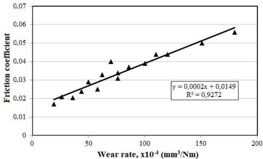
Figure 8. Relationship friction coefficient and wear rate on polymer composites
