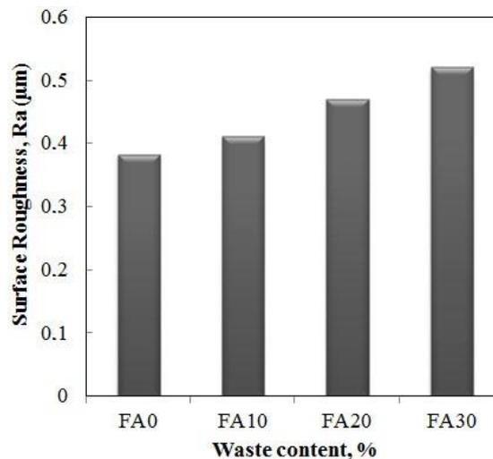
Figure 3. The variations in the surface roughness values of polymer composites with fly ash.
