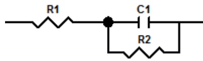
Figure 7: Equivalent circuit, used to fit measurement data obtained \text{LiMn}_2\text{O}_4 and Ni doped \text{LiMn}_2\text{O}_4 oxide pellets.
