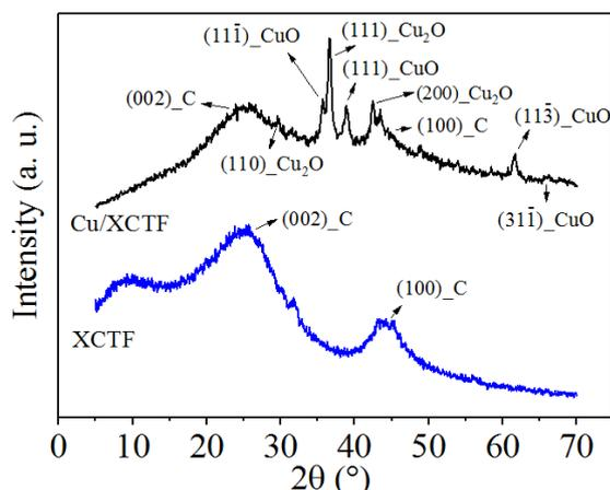
**Figure 1:** Diffraction patterns for XCTF and Cu/XCTF.
