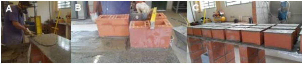
Figure 3: A) Mortar preparation, B) block levelling and C) capped blocks.
