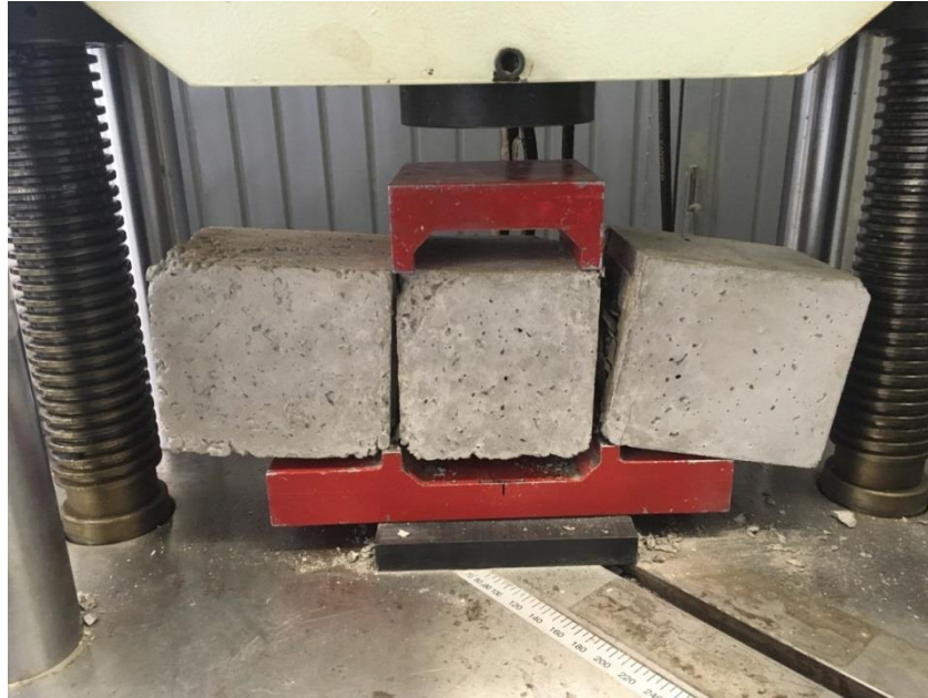
Figure 3: Shear failure of SCC specimen.
