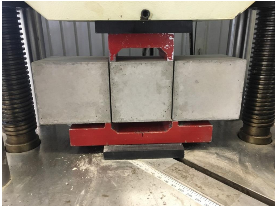
Figure 2: Concrete specimen and steel apparatus for direct shear test.
