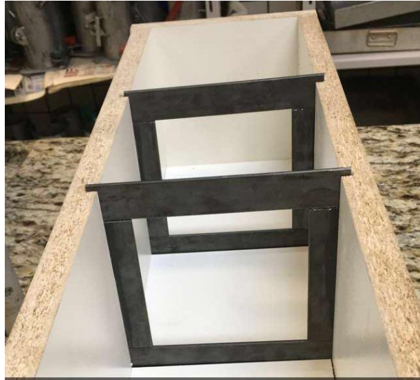
Figure 1: Prismatic specimens formworks.
