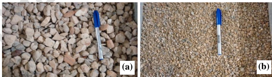
Figure 3: Recycled coarse aggregates a) D_{\text{max}} of 25.0 mm e b) D_{\text{max}} of 9.5 mm.
