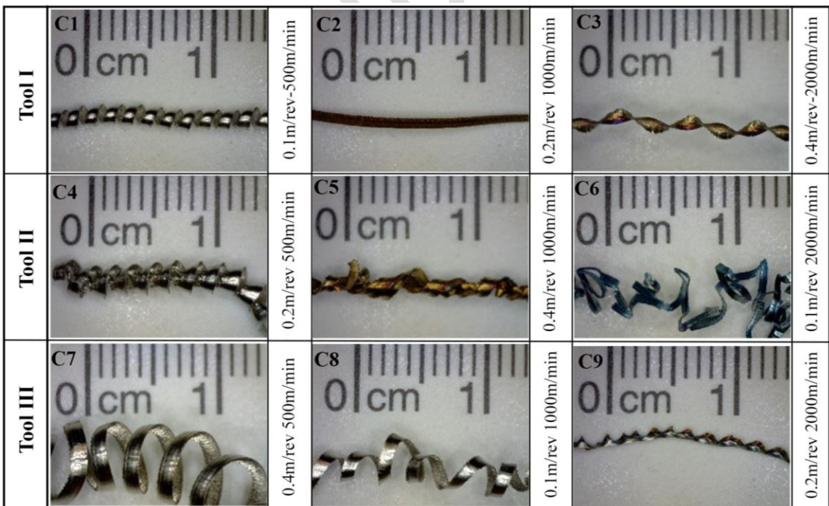
Figure 5. Chip formations at different face turning conditions
