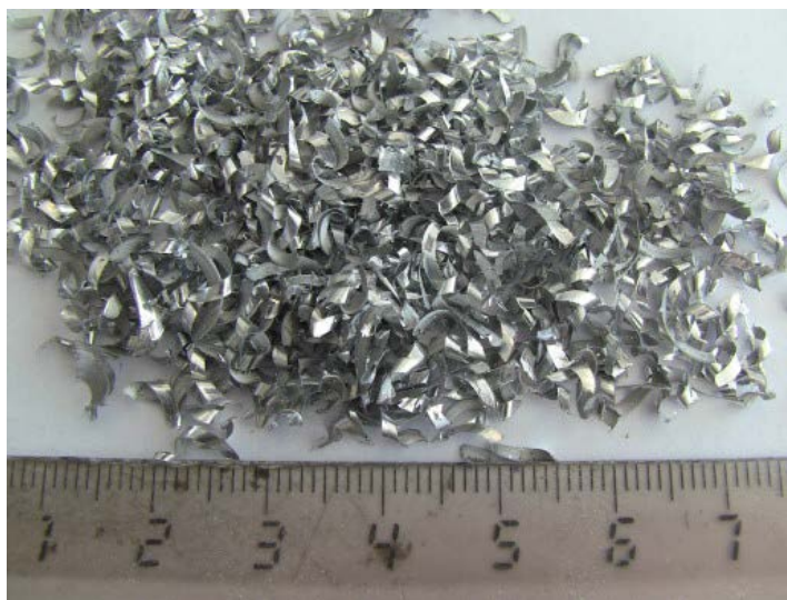
Figure 1: Chips of AA6013 alloy produced by CNC milling.
