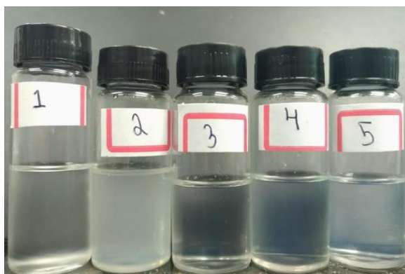
Figure 23 - Formulations in regions of liquid oil-in-water (points 1,2,3) and water-in-oil (points 4, 5) microemulsions.
