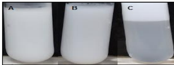
Figure 8 - A) Classification as gel macroemulsion in the proportion 6:4 after the fifth addition of salt water; B) Classification as viscous macroemulsion in the proportion 6:4 after the sixth addition of salt water; and C) Classification as phase separation in the proportion 6:4 after the seventh addition of salt water.
